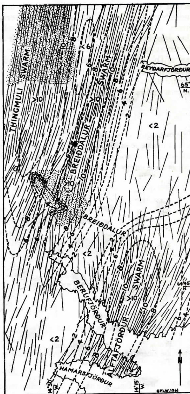
FIG. 8. Isopleths of the dyke-swarm, expressed as percentage dilation at sea-level. A few dykes are represented schematically to show the predominant trend. The three belts of high density each pass through a central volcano; the core of the Álftafjörður volcano lies several km south of the area of this map. *: Stafheidará exposure, where the dyke-swarm attains its maximum density of 20 per cent at sea altitude.
