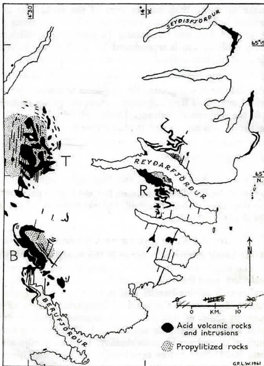
FIG. 2. The distribution of acid rocks in eastern Iceland (bedded acid tuffs in the flood-basalts omitted). The propylitized rocks in the cores of central volcanoes are also represented on this map. B : Breiddalur volcano; T : Thingmuli volcano; R : Reyðarfjörður volcano.
